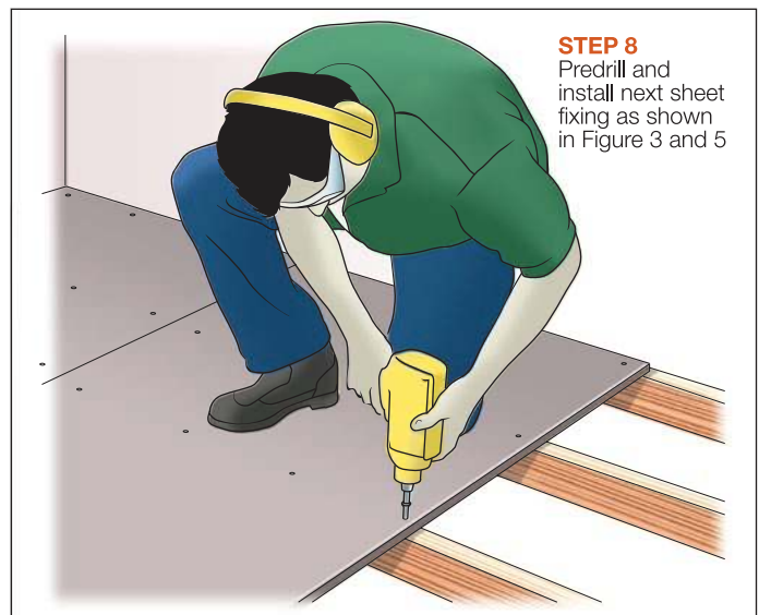
FIGURE 11 PRE DRILL NEXT SHEET
